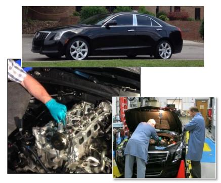
Cadillac ATS acquired. Instrumented cylinder head installed to support combustion analysis
