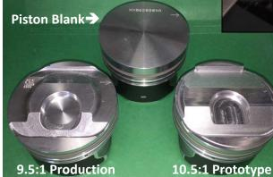
Pistons designed by Kolbenschmidt. Engine modeling/design guidance from GM. Blanks provided by Kolbenschmidt, machined in Oak Ridge
